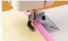
Piping / zipper foot
